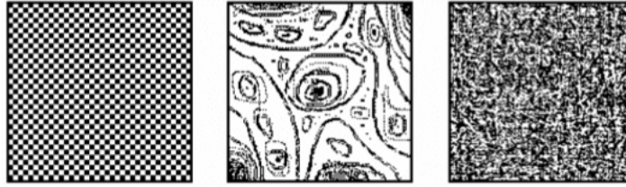
Figure 3.2: Three decorrelated signals: a complete ordered signal, a complex signal and white noise.
