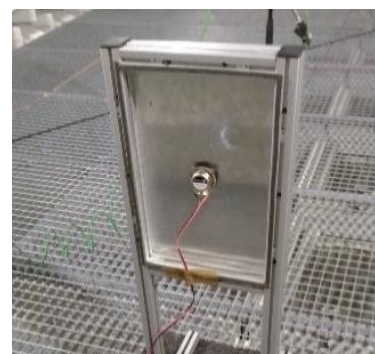
Figure 4: A collocated pair of actuator and sensor mounted on a thin clamped aluminum plate in an anechoic chamber. Dimensions: 28.5 cm * 43 cm * 1.5 mm
