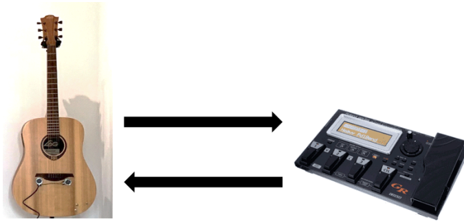
Figure 1: test of the hexaphonic HyVibe Guitar using a Roland GR 55 guitar synthesizer
