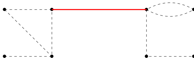
FIGURE 2.7 – Graphe contenant un isthme
